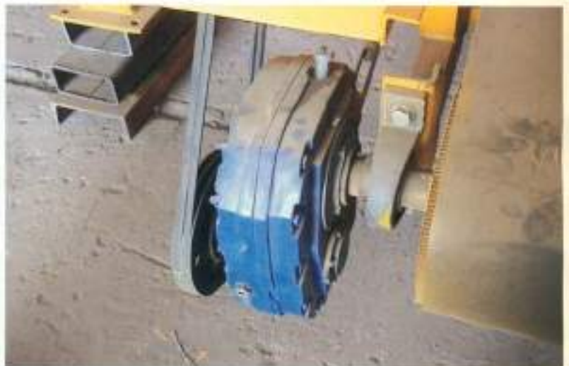
SMSR on a Conveyor Belt Drive
